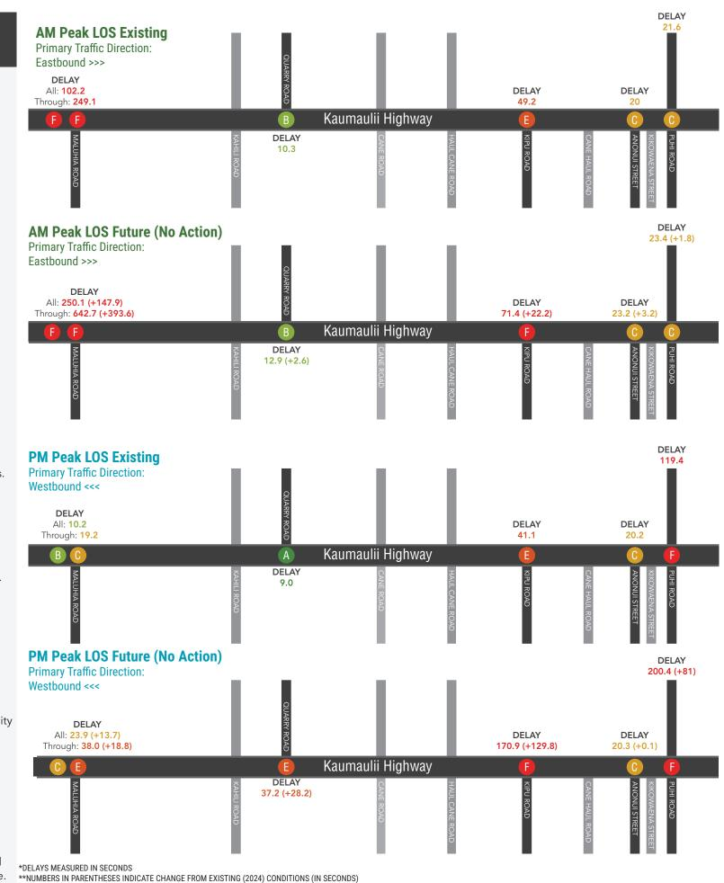
NOTE: FOR SIDE-STREET STOP-CONTROLLED INTERSECTIONS (QUARRY, KIPU, ANONUI), DELAY IS REPORTED FOR THE MOVEMENT WITH THE WORST SIDE-STREET DELAY. FOR SIGNALIZED INTERSECTIONS (PUHI), DELAY IS THE AVERAGE FOR ALL MOVEMENTS. AT MALUHIA, BOTH THE AVERAGE INTERSECTION DELAY AND THE HIGHEST MOVEMENT DELAY (EB THROUGH AM, WB LEFT PM) ARE SHOWN DUE TO UNIQUE CONGESTION.
